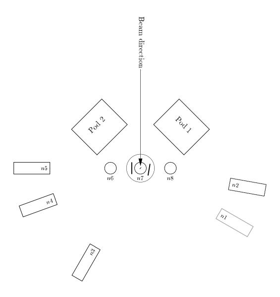
FIG. 1. A schematic of the layout of the various detectors around the target. The DEMON detectors are indicated by n1-n8. The n1 detector is below the reaction plane defined by the fission fragment detectors, while n2 and n6-n8 are above. The two pods of BaF<sub>2</sub> detectors are also shown. The two PPACs are indicated by the thicker straight lines between n6, n7, and n8. The reaction chamber is indicated by the thin-lined circle surrounding the target and PPAC's.
